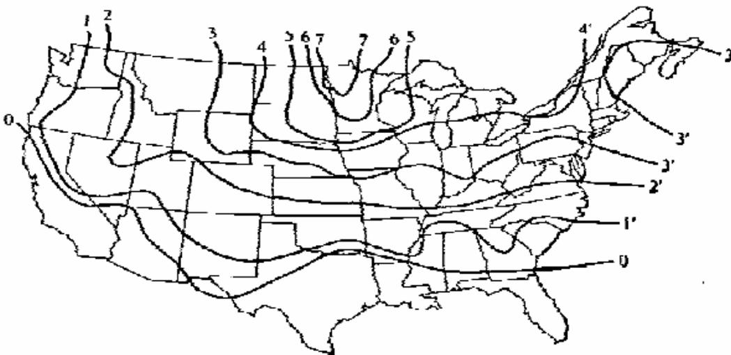
Figure1. Frost depth contours in the United States
